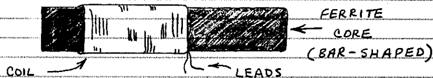
TYPICAL ANTENNA COIL
